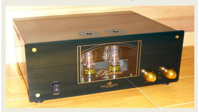
Ken Shindo's statement pre-amplifier. What can one possibly say about this pre-amplifier that could even begin to touch on it's virtues? High quality, custom wound output transformers are used. Moving magnet and moving coil inputs are included. Moving coil is via a built in balanced amorphous core step up transformer. Line stage is based around the amazing Western Electric 349A vacuum tube. Nothing can prepare you.
